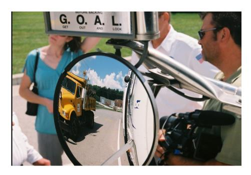
This picture, taken from the driver's seat, shows the left side spot mirror which helps the driver to see the vehicles in the left "No Zone" without that mirror the vehicle in the "No Zone" will disappear from view.
