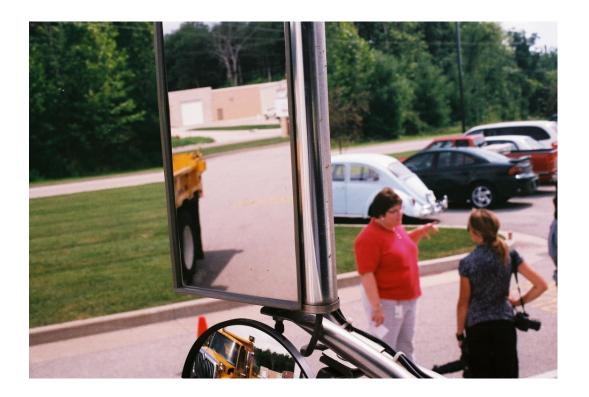
This picture shows what the driver can see when in the driver's seat and the advantage that the smaller mirror (spot mirror) gives the driver to locate vehicles in the left side blind spot. In the picture below a driver is explaining the no zone areas of the vehicle to one of the Institute's attendees.
